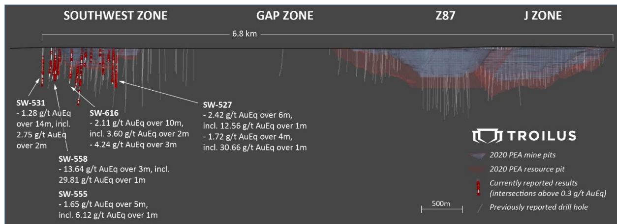
Figure 1. Long section Southwest > J Zone showing today's drilling at SW
